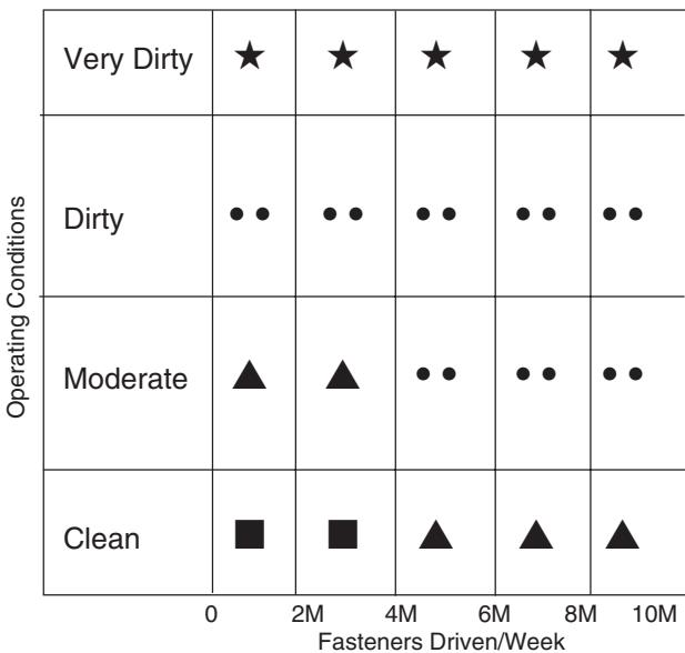
The maintenance interval for cleaning the **Duo-Fast Cordless Framing Nailer** will vary depending upon the number of nails driven per week, and the operating conditions under which the tool is used.
